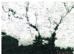
Example of trans-crystalline stress corrosion cracking on stainless steel 1.4401 with high chloride concentration.
